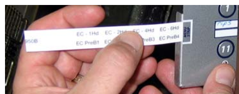
Figure 3: Removing menu strip.
