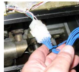
Figure 6: Attach fryer harnesses to supplied controller harnesses
