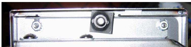
Figure 4: Removal of tinnerman clips may be necessary for proper fit.
